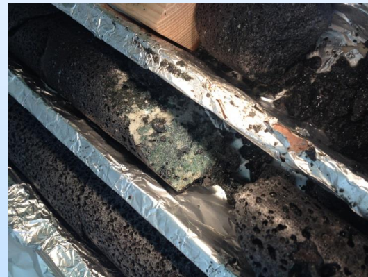
Calcite in a core retrieved from the site of the 2012 CarbFix injection of CO 2 -rich water into basalt in Iceland.
